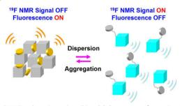
We report the multi-functionalized cubic silses quioxane (POSS) as the ratiometric multimodal chemosensors for monitoring solvent polarity with fluorescence and  $^{19}{\rm F}$  NMR.
